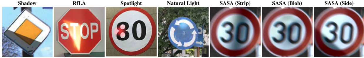
Figure 1. Light-based physical attacks on traffic signs: shadow casting [29], reflected laser [26], spotlight [28], and natural illumination [13]. The last three columns show SASA’s Strip, Blob, and Side shadow variants on the same sign.
